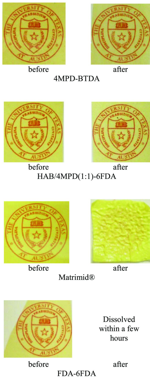
Figure 10. Photographs of some polymer films before and after benzene exposure in a Soxhlet extractor. Specific exposure times for each material are given in Table 5.
